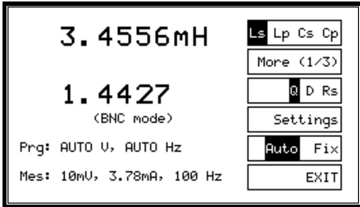
The upper measurement is that of the parameter selected by the 1st (upper) softkey. In this case, Ls, the series equivalent inductance, is 3.4556mH.
