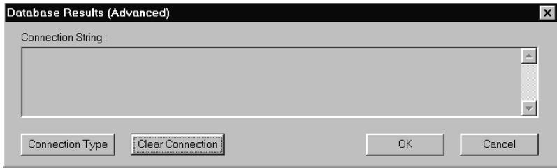
To connect to your database, the Server software uses a connection string that contains (amongst other things) the name of a provider, the name and location of the database and a valid database user name and password (if required). You may need to consult with the database or network administrator to obtain this information.
