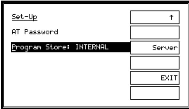
4. If, as shown above, the origin is INTERNAL, then press the softkey 'Server', so that the third line reads as follows:
